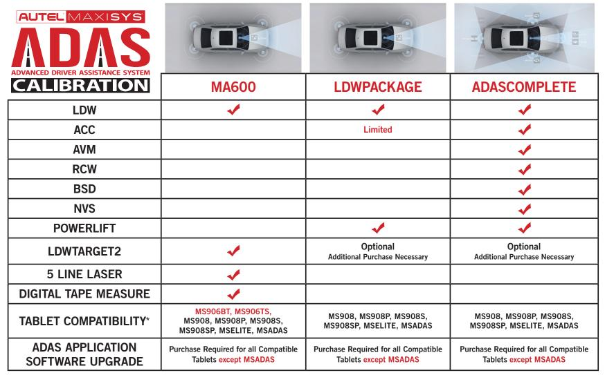
Tablet not included. The MA600 is compatible with the following tablets: MS906BT, MS906TS, MS908, MS908S, MS908SP, MSELITE and MSADAS. All tablet models require an additional one-time purchase software application upgrade, except MSADAS. Tablets with previously active ADAS application software will not be compatible with MA600.
